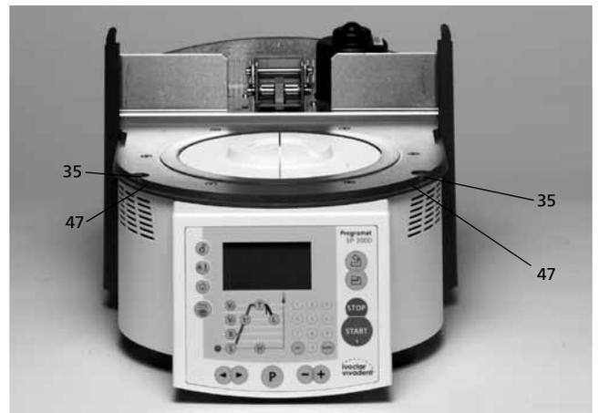
Place the cooling tray (34) on the frame plate (7).
