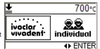
The cursor position (frame) can be changed by means of the Cursor keys. The marked type of press program can finally be selected using the Enter key.
