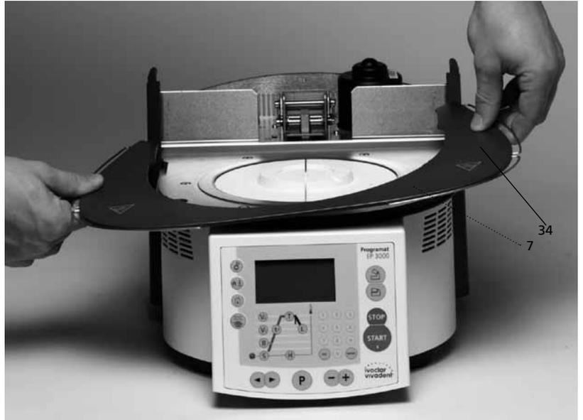
Secure the cooling tray (34) with the two screws
