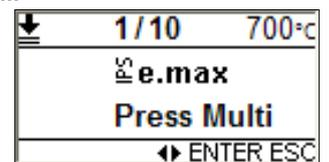
The Cursor keys can be used to toggle between the possible press programs. The displayed press program can finally be selected using the Enter key. The ESC key can be used to change to the selection of press program types.
